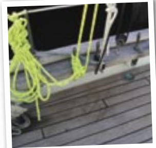
Modern lines on trad pin-rail
